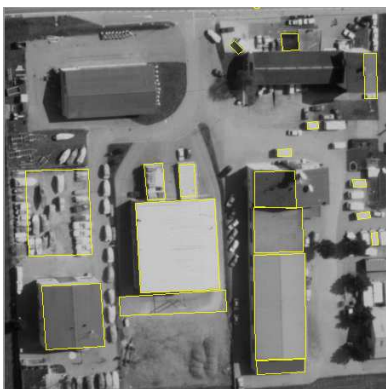
Figure 9: The input regions from the Avenches data set. The regions were obtained by running the Ascender I system.
