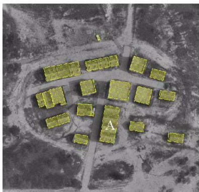
Figure 10: The input regions from the Fort Benning data set. These regions were obtained by a combination of polygons extracted using Ascender I and polygons extracted from SAR data.
