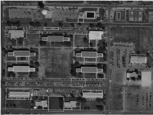
Figure 8: The input regions from the Fort Hood data set. These regions were obtained by running the original Ascender I system constrained to detect two-dimensional building footprints.
