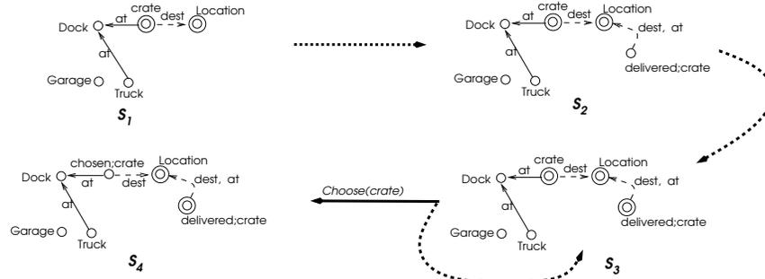
Figure 4: A loop in the belief state space of the delivery domain that makes progress in the concrete state space. The dotted edges represent a sequence of actions delivering one crate: Choose(crate), Load(), SenseAndSetDest(), Drive(), UnLoad(), SetDrivingDest(Dock), Drive().
