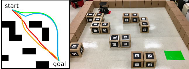
Figure 3: The OFFICE map (left) and the environment (right). The riskiest path (red), a very risky path (yellow), a very safe path (blue), and the safest path (green) are also shown.
